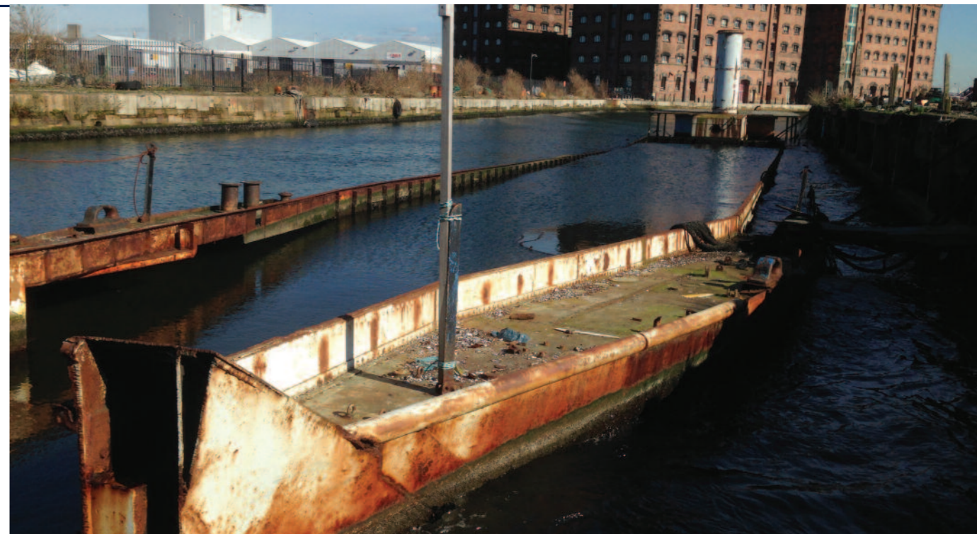
Above: LCT 7074 underwater, but with her 37 metre hull and the remains of a landing ramp still visible. This shows the size of these landing craft which could carry up to 11 tanks.
